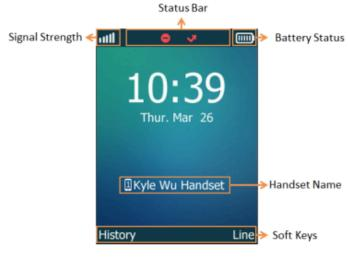
The LCD screen is divided into three parts: Status Line, Text Line and Softkey Line.
